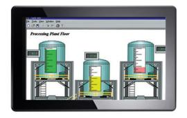
enclosure, fanless operation and protection against harsh environments and fluctuating temperatures are required. For the I/O interfaces, the same Ethernet, USB and serial ports as well as audio and additional monitor connectors are important — along with storage capabilities and expansion slots for additional functions and customization.
